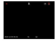
The state of image mirroring is indicated by the orientation of the "R" graphic at the center top of the display screen. In System Settings or Play-Back mode, use the *Up/Mirror* button to navigate menus
