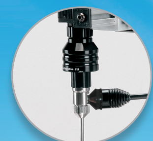
With a borescope (with optional VC-35 Video Coupler)
